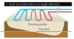
. Fluid circulation flow using the "Smart Thaw System".
